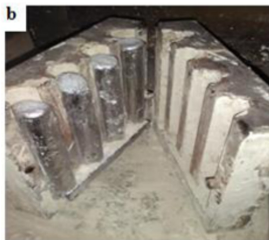
Fig. 1. (a) Pouring of molten metal into the die; (b) Removing of cast composite from die.
