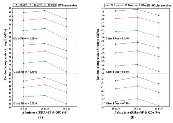
Fig. 2. (a) Residual compressive strength versus RHA, SF, and QD portions for diverse GFRTBC mixes cured in HCl; (b) Residual compressive strength versus RHA, SF, and QD portions for diverse GFRTBC mixes cured in H2SO<sub>4</sub>.
