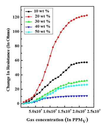
Fig. 7. Change in resistance with increase in the concentration of LPG of PANI/  $\text{ZnWO}_4$  composites.
