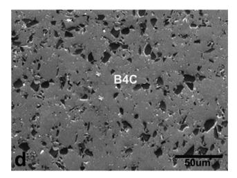
Fig. 2. SEM micrographs showing the distributions of particles in Al-7075/B\_4C composites with B\_4C.
