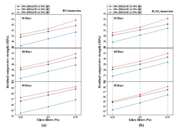
Fig. 3. (a) Residual compressive strength vs. glass fiber proportions for diverse GFRTBC mixtures cured in HCl; (b) Residual compressive strength vs. glass fiber proportions for diverse GFRTBC mixtures cured in H<sub>2</sub>SO<sub>4</sub>.
