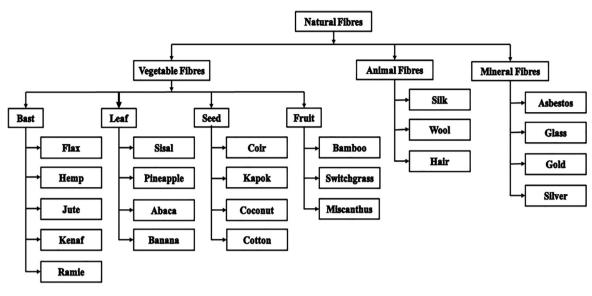
Fig. 1. Classification of Natural fibers reinforced composites [24].
