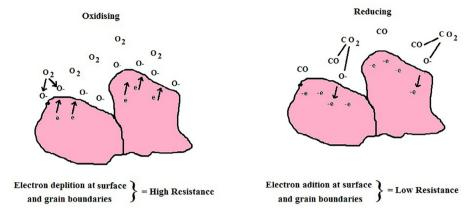
Fig. 1. Working principle of gas sensors in solid sensing material.
