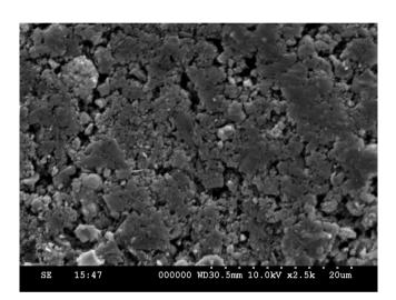
Fig. 5b. SEM image of PANI / ZnWO<sub>4</sub> composite.
