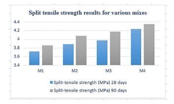
Fig. 4. Split-tensile strength at 28, and 90 days of curing.
