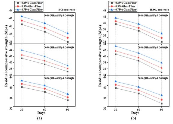
Fig. 4. (a) Residual compressive strength vs. periods curing for diverse GFRTBC mixtures cured in HCl; (b) Residual compressive strength vs. periods curing for diverse GFRTBC mixtures cured in H2SO4.
