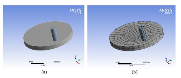
Fig. 3. (a) 3-D model of pin on disc in a wear testing; (b) Meshed Finite Element Model of pin on disc.
