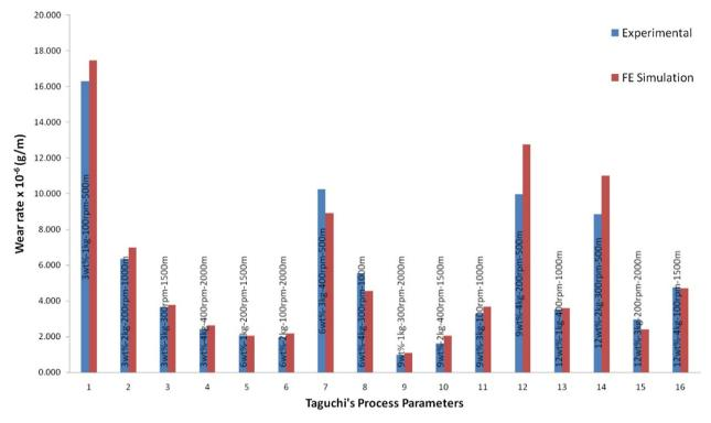
Fig. 4. Comparisons of FEM results with the experimental results.
