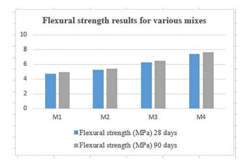
Fig. 5. Flexural strength at 28, and 90 days of curing.
