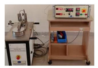
Fig. 1. Pin-on-disc tribometer.
