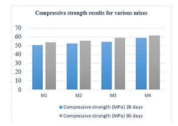
Fig. 3. Compressive strength at 28 and 90 days of curing.
