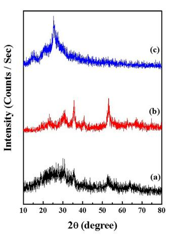
Fig. 4. X-ray diffraction pattern of (a) Pure PANI; (b) Pure ZnWO<sub>4</sub>; (c) PANI / ZnWO<sub>4</sub> composite.
