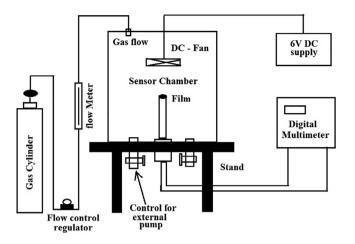
Fig. 2. The block diagram of the sensor setups used Gas sensing.
