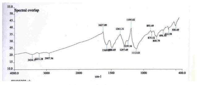
Fig. 3b. FTIR Spectra of PANI / ZnWO<sub>4</sub> composite.
