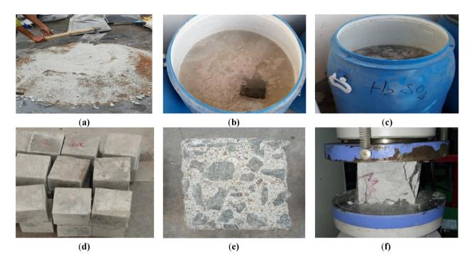
**Fig. 1.** (a) Mixing; (b) Curing samples in HCl solution; (c) Curing samples in H<sub>2</sub>SO<sub>4</sub> solution; (d) Sample following 90 days of HCl cure; (e) Sample after ninety days H<sub>2</sub>SO<sub>4</sub> curing; (f) Following ninety days of HCl cure, testing and failure patterns of the sample examined.
