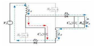
Fig.3.2. b equivalent circuits of mode 2
