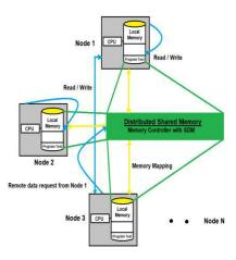
Fig 4. Architecture of distributed multi core architecture.
