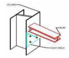
Figure 2. Column to Beam connection
