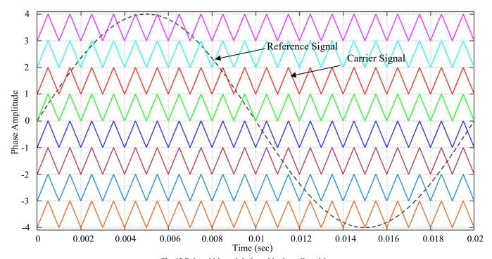
Fig. 12 Pulse width modulation with phase disposition
