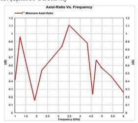
Fig 13. (e) Axial Ratio
