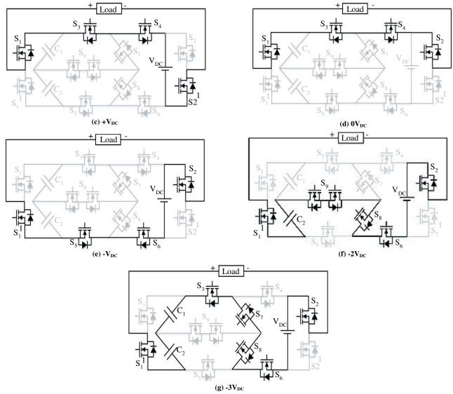
Fig. 3 Conduction paths of S<sup>3</sup>C7LBI for various voltage levels
