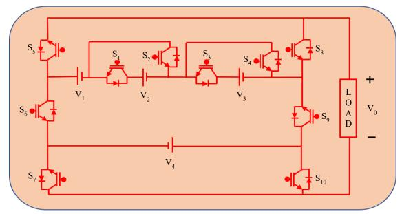
Fig. 2 Proposed nine-level multilevel inverter
