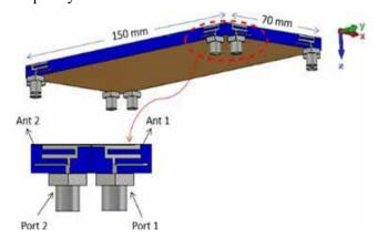
Fig. 1. Design illustartion of 8 x 8 Mimo antenna [15]
