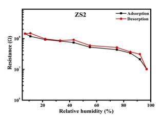
Fig. 14. Humidity hysteresis characteristic curve of calcinated Zn-SnO<sub>2</sub> NPs.
