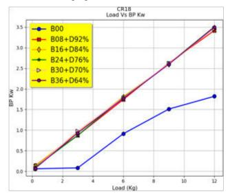
Figure 5: Load VS Break Power
