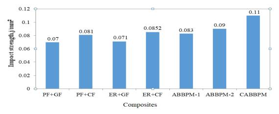
Figure 5.2 Bar chart showing Impact Strength with and Without Asbestos
