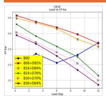
Figure 6: Load VS Friction Power
