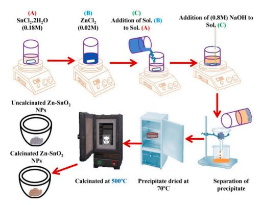
Fig. 1. Schematic representation for the synthesis of Zn-SnO<sub>2</sub> NPs by chemical coprecipitation method.
