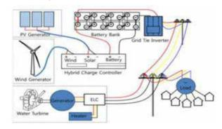
Fig. 8 A typical hybrid micro-hydroelectric, photovoltaic, and wind system is shown
