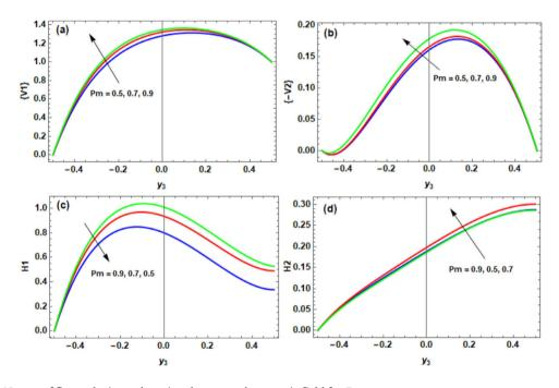
Nature of flow velocity and motional generated magnetic field for *Pm*.
