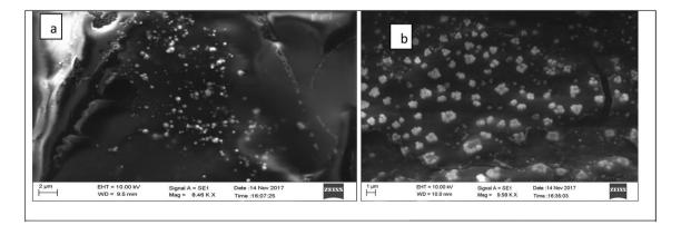
Fig. 5 SEM images of  ${\bf a}$  AgNPs and  ${\bf b}$  DMT-AgNPs
