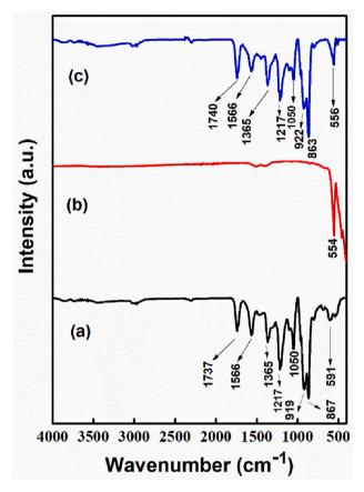
Fig. 5. Fourier-transform IR spectra of (a) PPy, (b)  $\mbox{Ho}_2\mbox{O}_3$  and (c) PPHO-3 composite.
