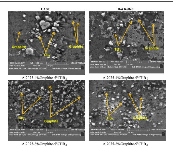
Fig. 5 SEM of Al7075/TiB<sub>2</sub>/graphite hybrid composites in Cast and Hot Rolled Conditions
