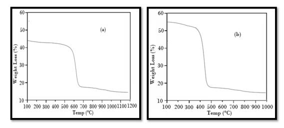
Fig. 7. TGA trace of (a) CuFe<sub>2</sub>O<sub>4</sub>(b) BaTiO<sub>3</sub> nanomaterials
