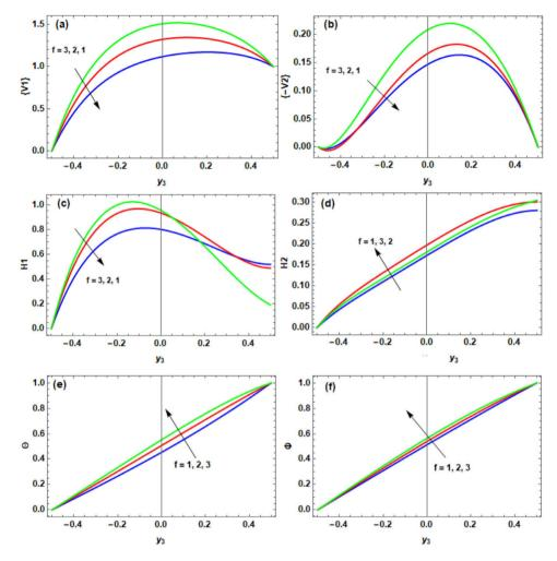
Nature of flow velocity, motional generated magnetic field, temperature field and concentration field for f.
