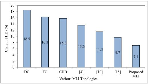
Fig. 21 Current analysis of proposed and conventional MLI
