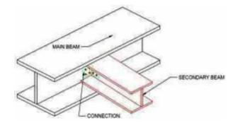
Figure 3. Beam to Beam connection
