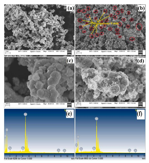
Fig. 4. FESEM images of Zn-SnO<sub>2</sub> NPs; (a, c) uncalcinated, (b, d) calcinated at 500 °C and EDS spectrum (e) uncalcinated, (f) calcinated at 500 °C.
