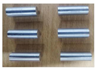
Fig. 4 Photograph of abrasive wear specimen
