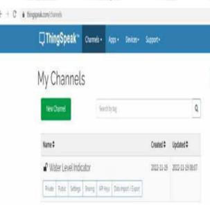
Now click on "API keys" tab and save the Write and Read API keys, here the use of only using "Write key". Get link as marked in the image which is need to "Copy" the key and link in the program.
