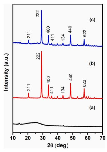
Fig. 4. X-ray diffraction spectra of (a) PPy (b)  ${\rm Ho_2O_3}$  and (c) PPHO-3 composite.
