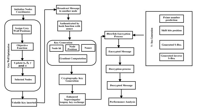
Figure 2: Proposed Scheme Block Diagram
