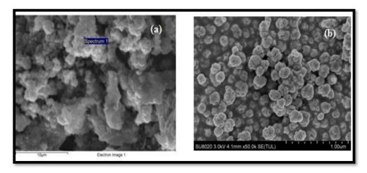
Fig. 5. SEM image of (a) CuFe<sub>2</sub>O<sub>4</sub> (b) BaTiO<sub>3</sub> nanomaterials
