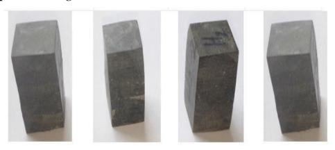
Figure 4.1 ASTM D-695 work pieces for compression test
