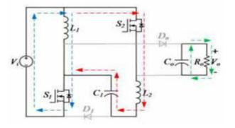
Fig.3.2. a equivalent circuits of mode 1
