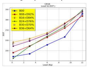
Figure 16: Load VS Exhaust Gas Temperature
