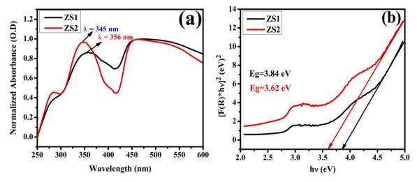
Fig. 7. UV-visible absorption spectra of synthesized Zn-SnO<sub>2</sub> NPs (a) Absorption spectrum (b) Kubelka-Munk plot of uncalcinated (ZS1) and calcinated (ZS2) NPs.
