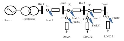
Figure 2. Single source 4-bus radial system
