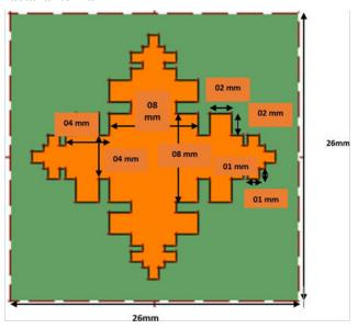
Fig 2. Detailed dimensions of a Minkowski Inspired fractal antenna
