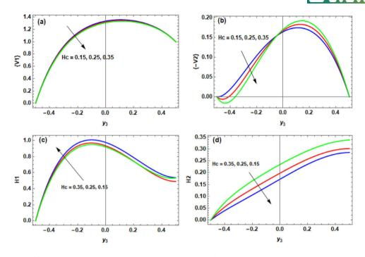
Nature of flow velocity and motional generated magnetic field for *Hc*.
