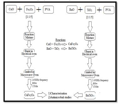
**Scheme 1.** Synthetic scheme of Copper ferrcopperd Barium titanate nanomaterials
