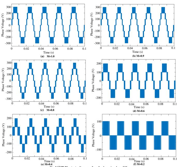
Fig. 5 S<sup>3</sup>C7LBI output voltage waveform for dynamic values of M
