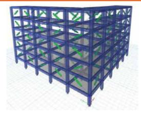
Fig. 7. 3D rendering of an atypical building with dampers
