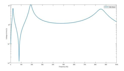
Figure 5. Voltage FRFof PZT-5H
