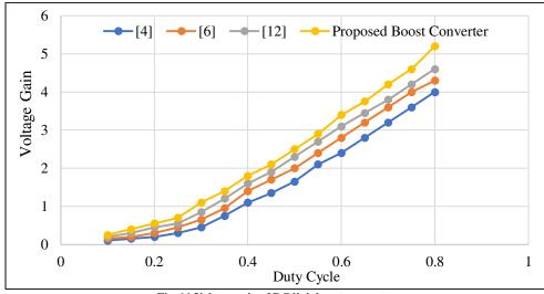
Fig. 11 Voltage gain of DC link boost converter
