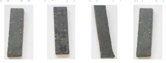
Figure 4.2 ASTM D-256 Work Pieces for Impact test
