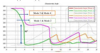
Fig 7. Characteristics Angle showing orthogonal modes
