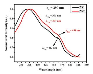
Fig. 8. Normalized emission spectra of the synthesized Zn-SnO $_2$  NPs; ZS1-uncalcinated and ZS2-calcinated at 500  $^{\circ}\text{C}.$
