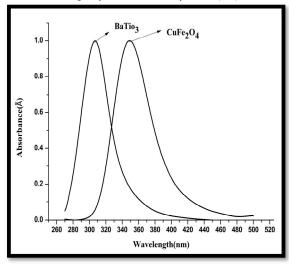
Fig. 8. UV-Vis spectra of CuFe<sub>2</sub>O<sub>4</sub> and BaTiO<sub>3</sub> nanomaterials
