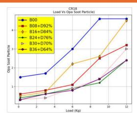
Figure 15 Load VS Smoke Opacity
