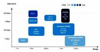
Fig. 2. Comparison of different WSN Technologies in terms of data rate, cost and range
