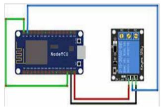
Fig 4: Interfacing of NodeMCU with Relay
