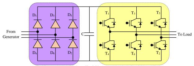
Fig. 2 Interconnection of diode rectifier-DC boost converter-three phase inverter to load
