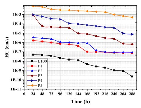
Fig. 10. Effect of HC with time on FA-EC blends permeated with DIW.
