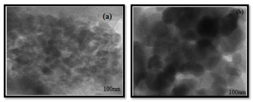
Fig. 6. TEM image of (a) CuFe<sub>2</sub>O<sub>4</sub>(b) BaTiO<sub>3</sub> nanomaterials
