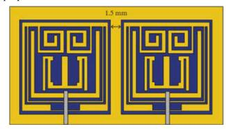
Fig. 8 Configuration of antenna [19]
