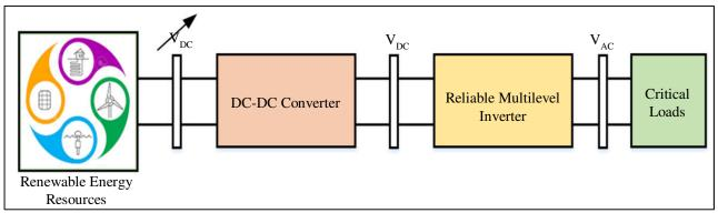
Fig. 1 Block diagram of integration of renewable energy resources to critical loads
