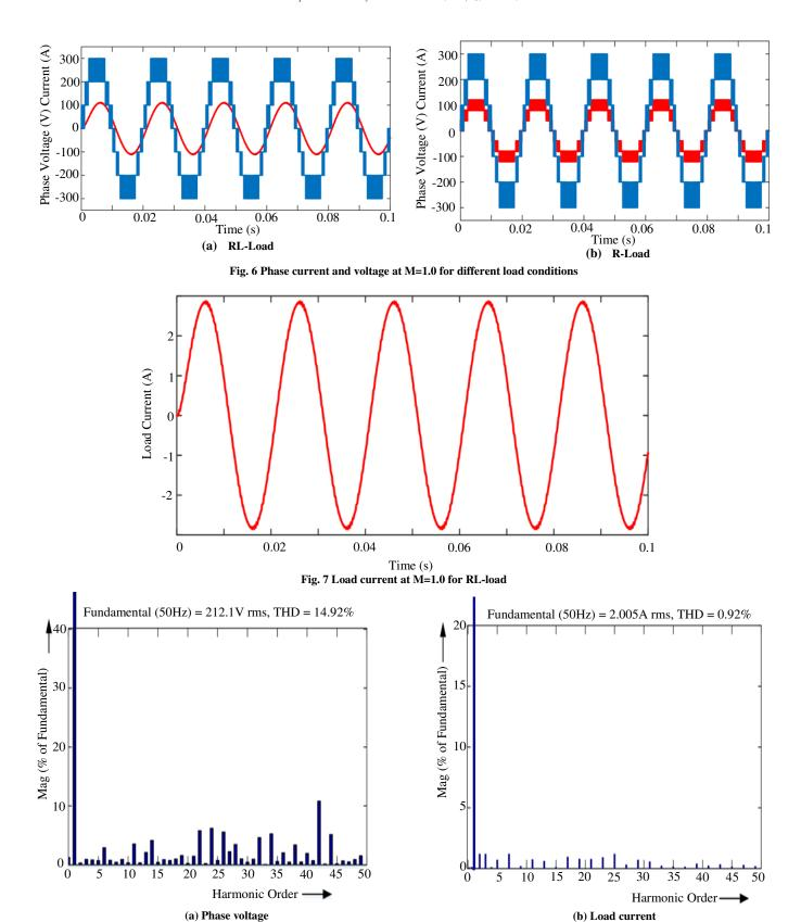
Fig. 8 Frequency spectra at unity modulation index
