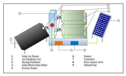
FIGURE1. Solar Photovoltaic assisted dryer Experimental setup
