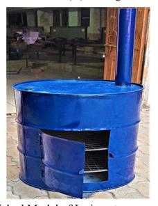
(vii) Finished Model of Incinerator
