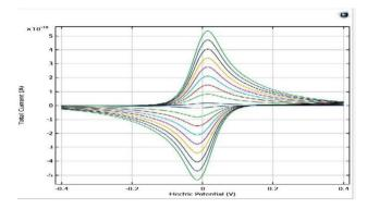
Fig. 12 Voltammetry plot of cylindrical electrode
