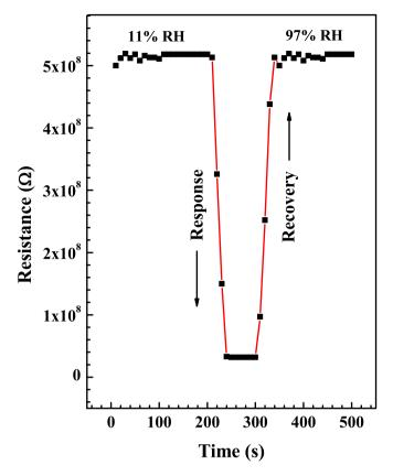
Fig. 11. Response and recovery plots of PPHO-3 composite.
