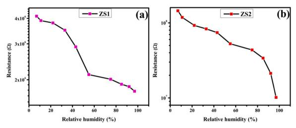
Fig. 10. Electrical resistance variation of Zn-SnO<sub>2</sub> NPs with different humidity conditions; for (a) uncalcinated (ZS1) and (b) calcinated at 500 °C (ZS2) NPs.
