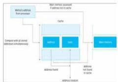
Fig.2 Architecture and data flow of a typical cache memory unit.
