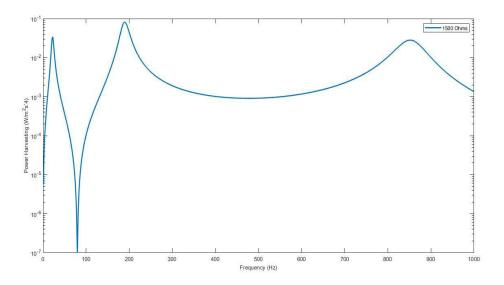
Figure 9.Power FRF of PZT-5H
