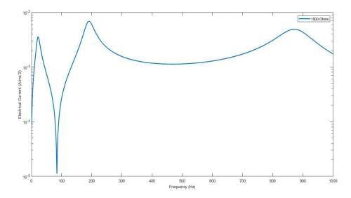
Figure 6.Current FRF of PZT-5A
