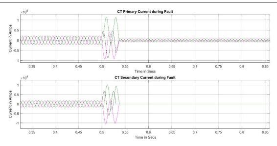
Figure 5. Fault current in primary side of CT for Relay 2 and 1 for fault point B
