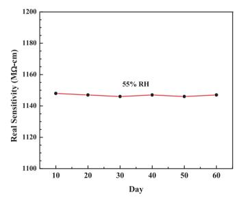
Fig. 13. Sensing stability of PPHO-3 composite.
