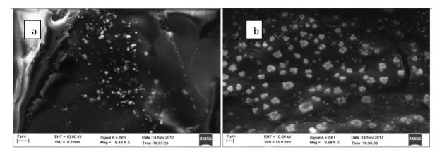
Fig. 5. SEM images of a) AgNPs, b) DMT-AgNPs.
