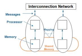
Fig. 3 Memory mapping Architecture using shared memory.
