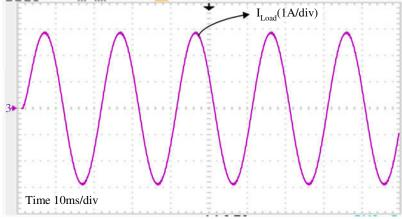
Fig. 10 Practical load current waveform at M=1.0
