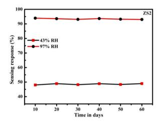
Fig. 15. Plot of stability testing of the calcinated Zn-SnO $_2$  NPs sensor for every 10 days at 43% RH and 97% RH.
