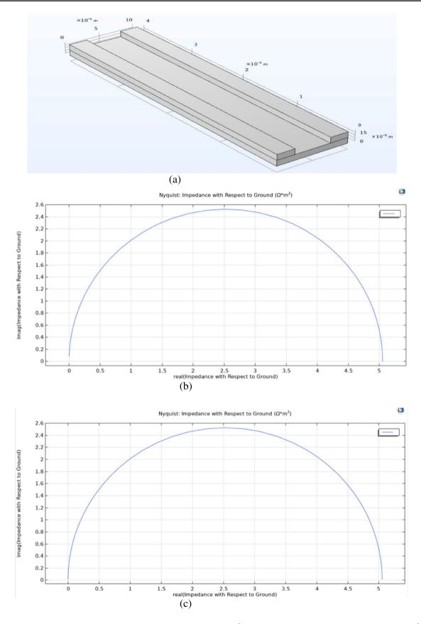
Fig. 6 a Cuboidal electrode. b Cuboidal electrode Nyquist plots for  $C_{\rm dl} = 20~\mu {\rm cm}^3$ . c Cuboidal electrode Nyquist plots for  $C_{\rm dl} = 100~\mu {\rm cm}^3$ .
