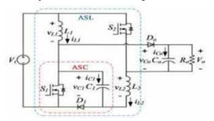
Fig.2.1 circuit diagram of ASLC converter
