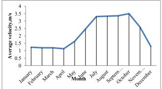
Figure 7. Average water stream flow velocity in each month
