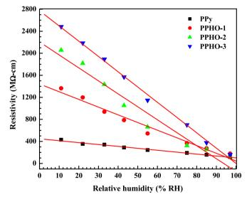
**Fig. 8.** Variation of resistivity with % RH for PPy and the composites. Solid lines are the best fits obtained from liner regression.
