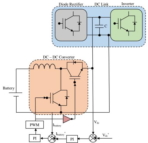
Fig. 3 Controller of DC-DC converter and diode rectifier and inverter system
