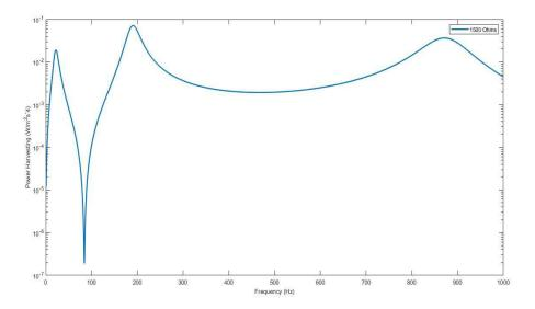
Figure 8.Power FRF of PZT-5A
