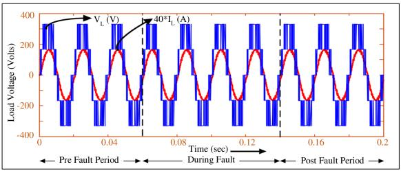
Fig. 8 Load current and load voltage waveforms for fault in S<sub>3</sub>
