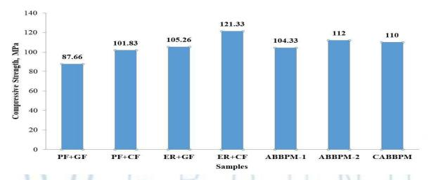
Figure 5.1 bar chart showing Compressive Strength – with and without Asbestos
