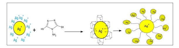
Fig. 1 Functionalization of AgNPs by 4-amino,3,5-dimercapto-1,2,4 triazole
