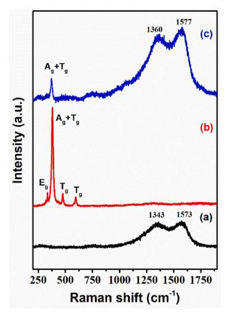
Fig. 7. Raman spectra of (a) PPy, (b) Ho<sub>2</sub>O<sub>3</sub> and (c) PPHO-3 composite.
