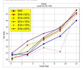
Figure 13: Load VS Hydrocarbon Emission
