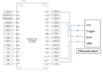
Fig 3: Interfacing of NodeMCU with Ultrasonic sensor
