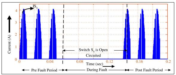
Fig. 10 Switch S<sub>4</sub> current waveform for fault in S<sub>4</sub>
