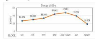
Figure 9: - Story Drift in Y direction for zone III
