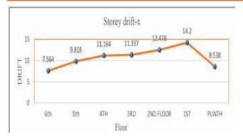
Figure 12: - Story Drift in X direction for zone IV
