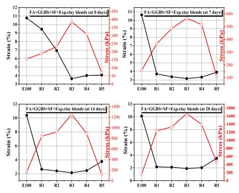
Fig. 9. Variation of stress-strain for FA-GGBS-SF-EC blends at various curing periods.
