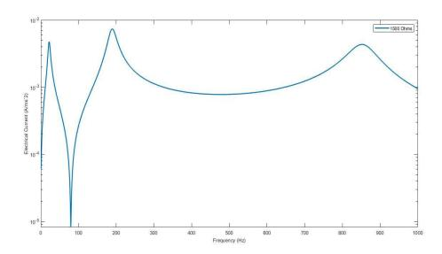
Figure 7.Current FRF of PZT-5H
