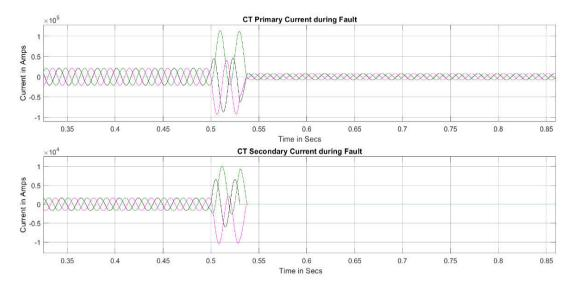
Figure 4. Fault current in primary side of CT for Relay 1 and 2 for fault point A
