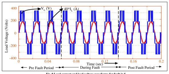
Fig. 9 Load current and load voltage waveforms for fault in S<sub>4</sub>
