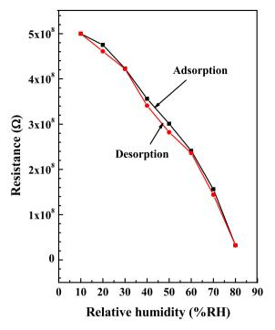
Fig. 12. Humidity hysteresis curve of PPHO-3 composite.
