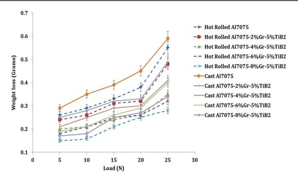
Fig. 9 Variations in weight loss of the cast and hot-rolled samples with different loads
