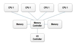
Fig 2. Memory controller Architecture.
