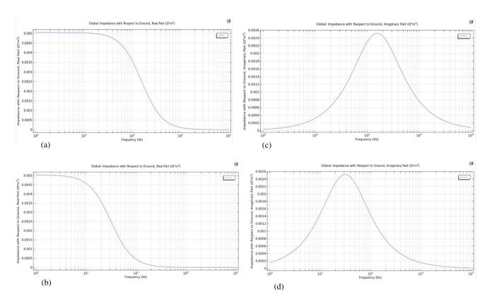
Fig. 5 a Stepped cuboidal electrode Bode—real impedance versus frequency plots for  $C_{\rm dl}$ =20  $\mu {\rm cm}^3$ . b Stepped cuboidal electrode Bode—real impedance versus frequency plots for  $C_{\rm dl}$ =100  $\mu {\rm cm}^3$ . c
