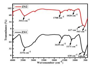
Fig. 6. FT-IR spectra of synthesized Zn-SnO  $_2$  NPs; ZS1-uncalcinated, ZS2- calcinated at 500  $^{\circ}\text{C}.$
