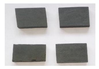
Figure 4.3 ASTM D-2240 Work Pieces for Hardness test
