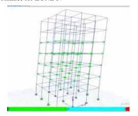
Figure 7: - Pushover examination of steel building performance for ZONE V
