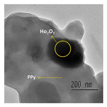
$\textbf{Fig. 6.} \ \ \textbf{Transmission electron micrograph of PPHO-3 composite}.$
