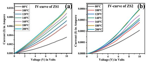
Fig. 9. Conductivity response of synthesized Zn-SnO<sub>2</sub> NPs at different operating temperatures ranging from 80 °C to 200 °C; (a) for uncalcinated (ZS1) and (b) calcinated at 500 °C (ZS2).
