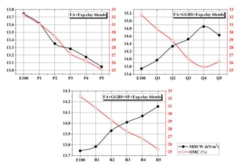
Fig. 5. Variation of MDUW and OMC of expansive clay blends.
