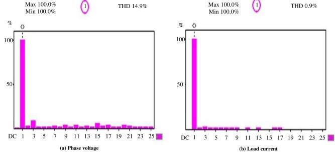
Fig. 11 Practical frequency spectra at unity modulation index
