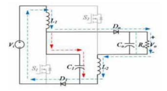
Fig.3.1.b equivalent circuit of mode 2
