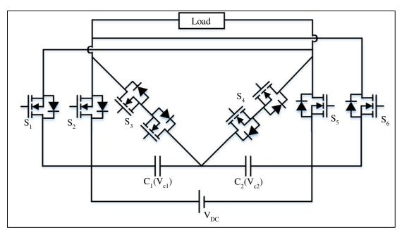
Fig. 2 Proposed Reliable Five Level Inverter (RFLI)
