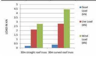
**Graph 1:- Loading At Each Node for Angle and Tubular Section**
