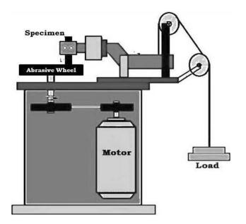
Fig. 2 Photograph of abrasive wear test setup
