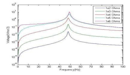
Figure 3.Plot of Voltage FRF
