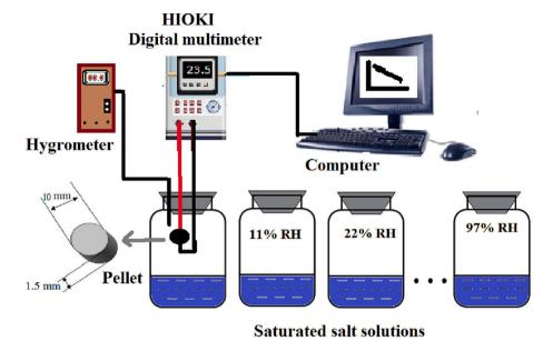
Fig. 1. Illustration of the humidity sensor set up for humidity sensing measurements.
