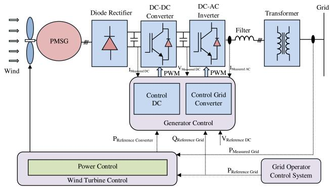
Fig. 1 Structure of isolated wind turbine conversion system
