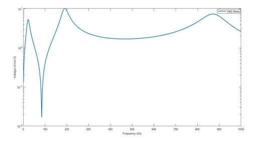
Figure 4. Voltage FRF of PZT-5A
