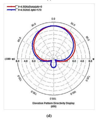
Fig 12. (a) Azimuth pattern gain display (b) Elevation pattern gain display (c) Azimuth pattern directivity display (d) Elevation pattern directivity display
