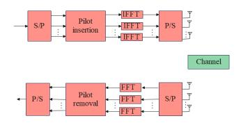
Figure 2. System model of MIMO-OFDM
