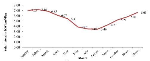
Figure 5. solar intensity KWh/m<sup>2</sup>/day available at the site for all the months
