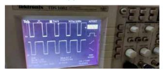
Fig.4.2 b Output of driver circuit
