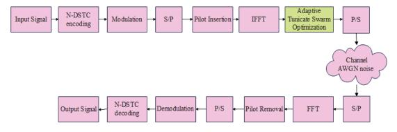
Figure 1. Workflow of the proposed method with MIMO-OFDM
