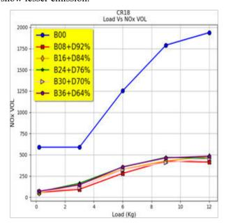
Figure 14: Load VS Nitrogen Oxide Emission Smoke opacity
