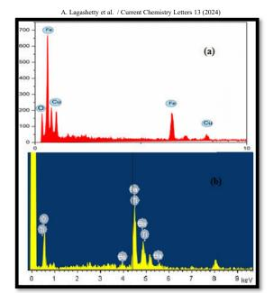
Fig. 4. EDX pattern of (a) CuFe<sub>2</sub>O<sub>4</sub> (b) BaTiO<sub>3</sub> nanomaterials
