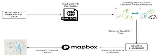
Fig. 1 Block diagram representing vehicle route optimization methodology
