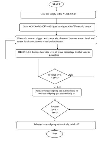
Fig 2: Flowchart of the proposed water monitoring and controlling system
