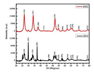
Fig. 3. The XRD pattern of synthesized Zn-SnO $_2$  NPs; ZS1 is uncalcinated, and ZS2 is calcinated at 500  $^{\circ}$ C.
