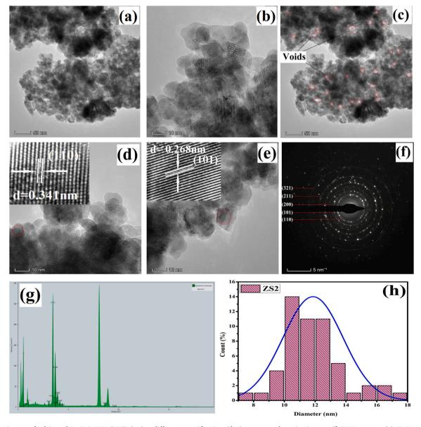
Fig. 5. TEM images of calcinated Zn-SnO<sub>2</sub> NPs (ZS2); (a-c) at different magnification, (d, e) represents d-spacing images, (f) SAED pattern, (g) EDAX spectrum and (h) particle size distribution histogram.
