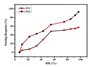
Fig. 11. Variation of sensing response of uncalcinated (ZS1) and calcinated (ZS2)  $\text{Zn-SnO}_2$  NPs with relative humidity.
