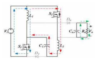
Fig.3.2.c equivalent circuits of mode 3
