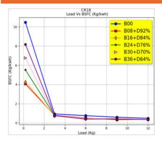
Figure 9: Load VS BSFC
