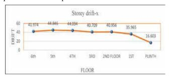
Figure 8: - Story Drift in X direction for zone III
