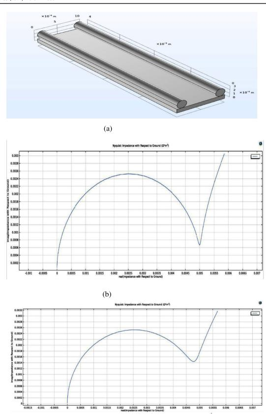
Fig. 8 a Cylinder electrode. b Cylinder electrode Nyquist plots for  $C_{\rm dl} = 20~\mu {\rm cm}^3$ . c Cylinder electrode Nyquist plots for  $C_{\rm dl} = 100~\mu {\rm cm}$ .
