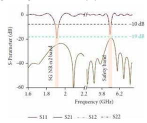
Fig. 9 Simulated results for reflection coefficient and isolation [19]
