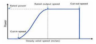
Fig. 11 Wind turbine power characteristics
