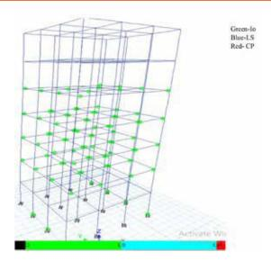
Figure 5: - Push over examination of steel building performance for ZONE III
