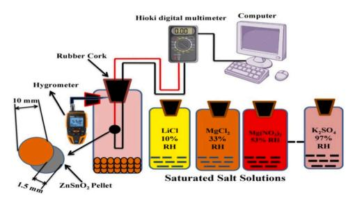
Fig. 2. Schematic diagram of the humidity sensing set up.
