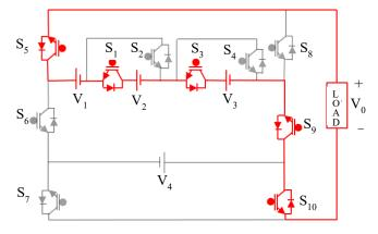
Fig. 4 +3V<sub>DC</sub> output voltage
