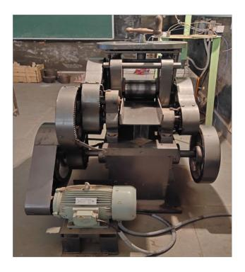
Fig. 1 Photograph of hot rolling machine
