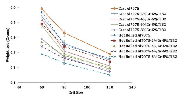
Fig. 11 Variations in weight loss of the cast and hot-rolled samples with different grit size
