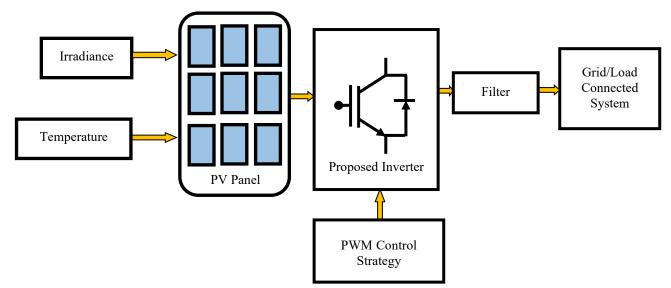
Fig. 1 PV interconnected modified MLI
