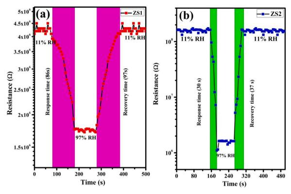
Fig. 13. Plot of response and recovery time of synthesized  $Zn-SnO_2$  NPs sensor with change in relative humidity; (a) Uncalcinated (ZS1) (b) Calcinated (ZS2)  $Zn-SnO_2$  NPs.
