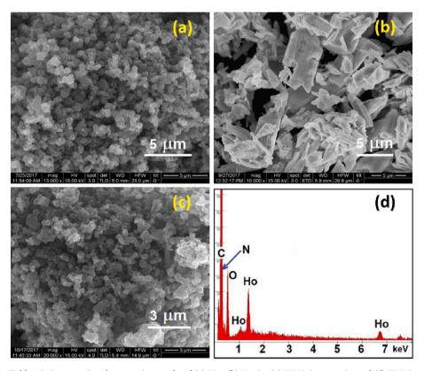
$\textbf{Fig. 2.} \ \ \text{Field emission scanning electron micrographs of (a) PPy, (b) Ho}_{2}O_{3}, (c) \ PPHO-3 \ composite \ and \ (d) \ EDX \ Spectrum.$
