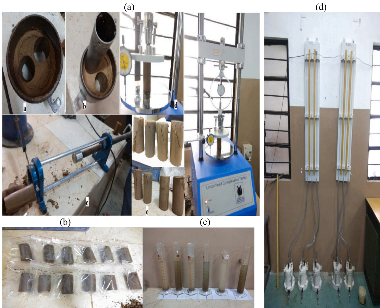
Fig. 2. (a) UCS testing of soil samples (Compaction of specimen to MDD and OMC, Inserting Sampler tube, Extraction of specimen to standard dimensions, Compression testing) (b) UCS samples stored in polythene bag for curing (c) FSI test (d) Hydraulic conductivity test.
