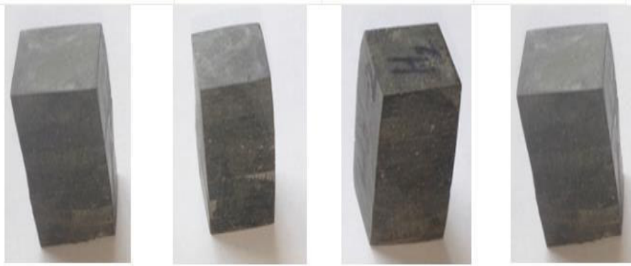
Figure 4.1 ASTM D-695 work pieces for compression test
